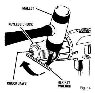
Open chuck jaws and remove wrench. Remove the chuck screw by turning it in a clockwise direction. See Figure 15. Note: The screw has left hand threads.
